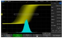
Waveform and measurement histograms (standard)
