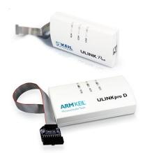
The Keil ULINK family of debug and trace adapters connects the host computer via USB to your target system. ULINK uses on-chip debug interfaces and supports application debugging and flash programing.
